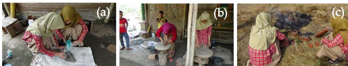
Figure 1. Making teapots with the addition of zeolite and activated charcoal (a) Ingredients formulation (b), Forming a clay pot, (c) Burning clay teapot
