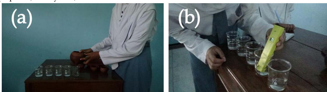
Figure 2. Trial of the teapot using sea water Trial of the teapot using sea water (a) Water clarity test and (b) pH testing
